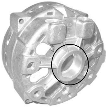
PX-2/4 rear housing is shorter in rear bearing area than a PX-5. New-style castings with extra holes will replace all earlier style using a clip-retained rear bearing. PX-1124 Housing, Rear, Bare (PX2&PX4G-5)
